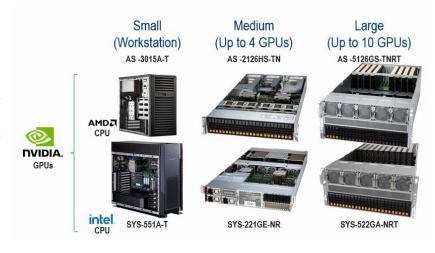
Supermicro offers the following choices to support up to **8 NVIDIA L40S or RTX GPUs** to run Ansys physics solvers and NVIDIA Omniverse. NVIDIA H100/H200 GPUs could be used to run Ansys physics solvers.
