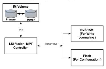
Figure 4-1. Typical Integrated Mirroring Implementation
