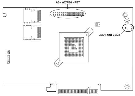
Figure 2-2 displays LED indicators on the add-on card, while table lists the individual LEDs, their state and their specification.
