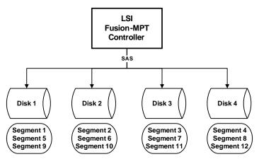
Figure 5-1. Integrated Striping Example
