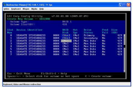
4. Move the cursor to the RAID DISK column and select a line that has a **No** entry in this column, indicating that the disk is not already part of the volume being created. To add the disk to the new volume, change the No to **Yes** by pressing the space bar.
