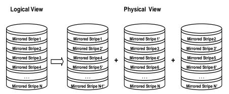
You can configure an Integrated Mirroring and Striping volume with an even number of disks, ranging from four minimum to ten maximum. Figure shows the logical view and physical view of an Integrated Mirroring and Striping volume with four mirrored disks. The firmware writes each mirrored stripe to a disk and mirrors it to an adjacent disk. RAID 10 is another term for this type of mirrored/striped configuration.
