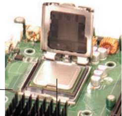
CPU in the CPU socket
