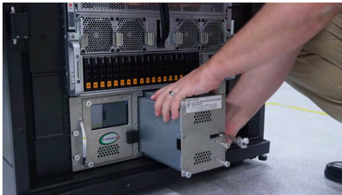
Patrick Removing A Supermicro CDU Pump
