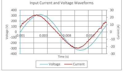
Input AC Current Waveform (ITHD = 4.64%, 50% Load)
