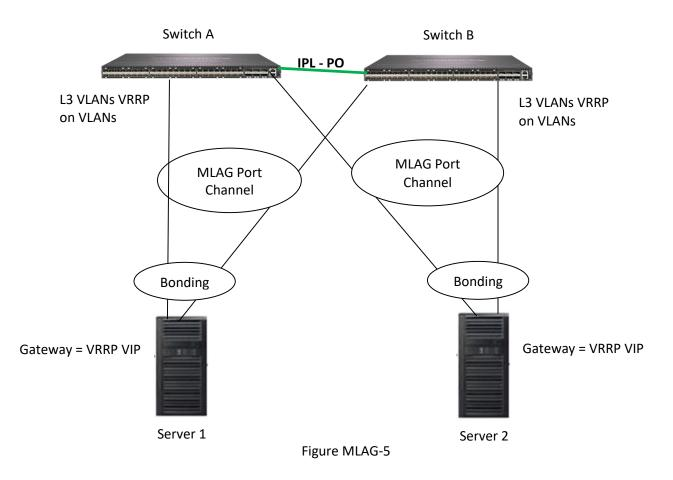
In Figure MLAG-5 Switches A and B are peer switches in the MLAG. Switches A and B are connected through an IPL port channel interface.
