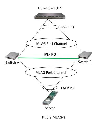
In Figure MLAG-3, Switch A and Switch B are peer switches in the MLAG. Switches A and B are connected through an IPL port channel interface.
