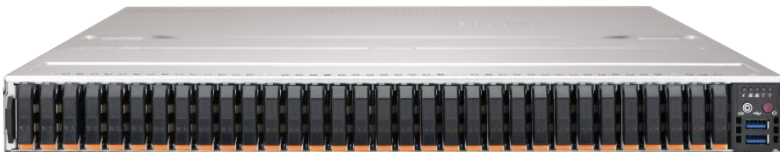
Image 4 - X11 Server with 32 x 5.9mm or 9.5mm E1.S
