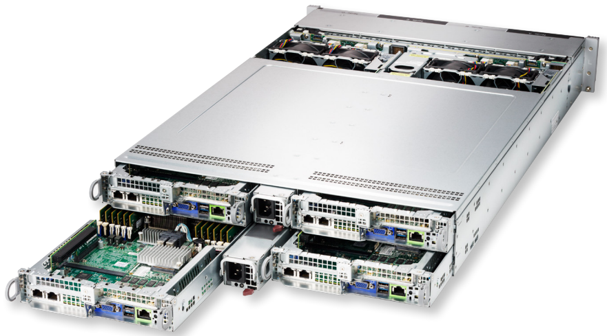
Figure 1. Supermicro 2U 4-Node BigTwin System (rear system view)
