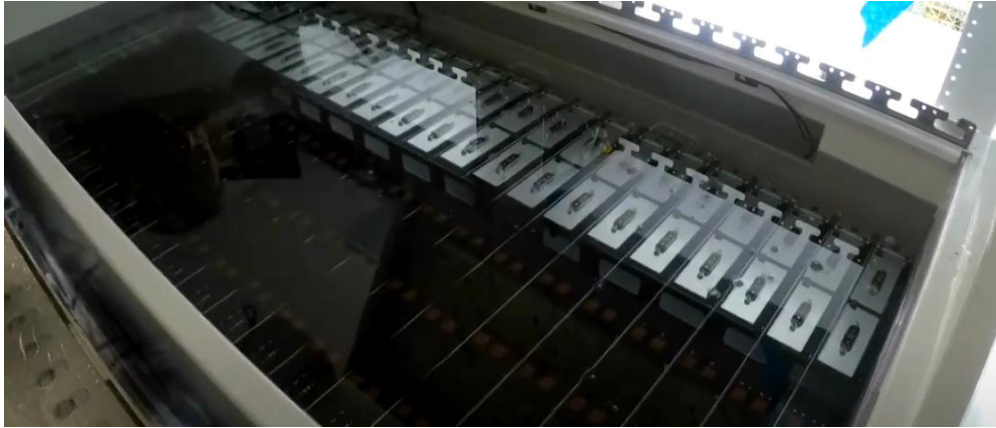
Figure 6 - Several Servers Immersed in Liquid
