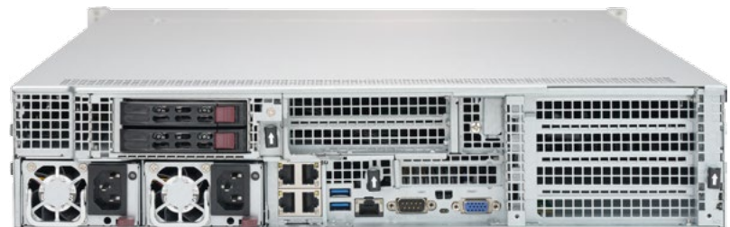
Figure 3. Supermicro 2U Ultra SuperServer 2028U-TN24R4T+: 24 NVMe drives is used to set a new performance record.
