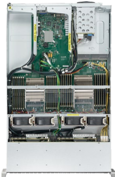
Figure 3. Supermicro 2U Ultra SuperServer 2028U-TN24R4T+: 24 NVMe drives is used to set a new performance record.
