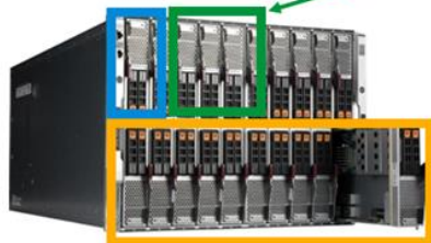
Supermicro SuperBlade 8U Enclosure
