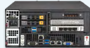
SYS-E403-13E-FRN2T 2x 2.5" hot-swap NVMe AC power supply
