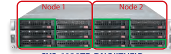
SYS-6028TP-DNC/(T)(F)R Up to 4x NVMe + 2x SAS 3.0 drives (per node), or Up to 6x SAS 3.0 support (per node)
