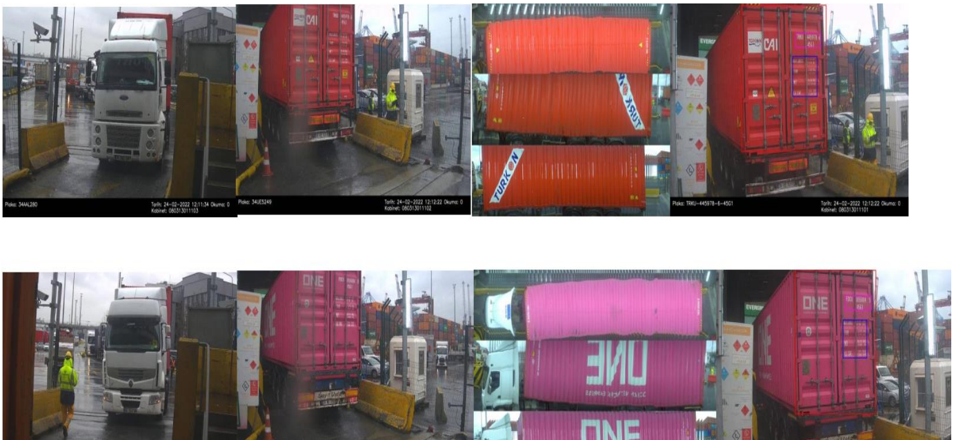
Figure 2 – The ConScan Container and Truck Identification Recognition and Tracking System Output
