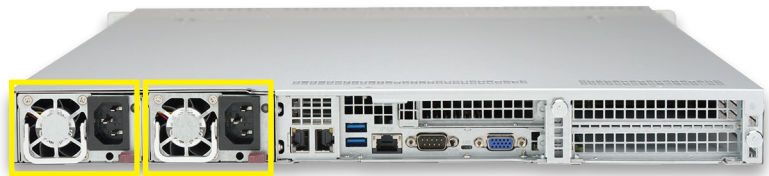
Figure 10. Low power consumption: 1000W Titanium Level (96%) Redundant Power Supplies.
